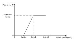
Figure 4.1: Production curve of a wind power unit.
