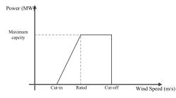
Figure 2.2: The production curve of a wind power unit
