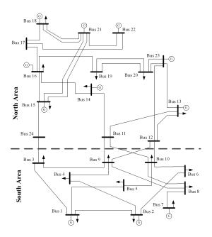
Figure 5.2: Single-line diagram of the the IEEE-RTS96.
