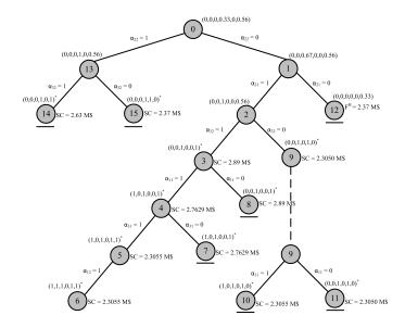
Figure 4.5: The branch-and-bound tree of the MBA for the 3-bus example system;  $(x,x,x,x,x,x)=(\alpha_{11},\alpha_{12},\alpha_{21},\alpha_{22},\alpha_{31},\alpha_{32}), \alpha \in \{0,1\}$ , SC: Social Cost.
