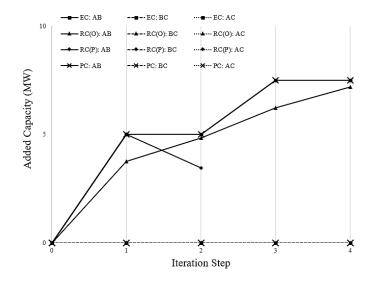
Figure 4.7: Development of added capacity to the lines during the iterations for the 3-bus example system with reduced generating capacity.
