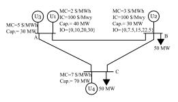
Figure 4.4: The 3-bus example system; MC: Marginal Cost, IC: Investment Cost, Cap.: Capacity, IO: Investment Options (in MW).
