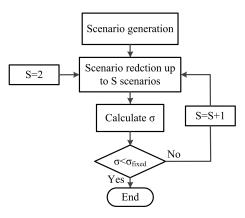
Figure 2.3: The flowchart of scenario-based modelling of each slot in horizon year of planning
