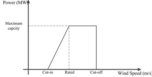
Figure 4.1: Production curve of a wind power unit.
