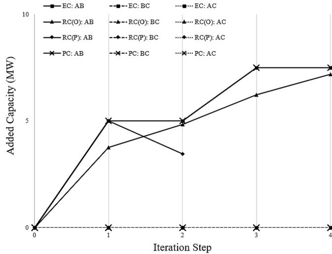
Figure 4.7: Development of added capacity to the lines during the iterations for the 3-bus example system with reduced generating capacity.
