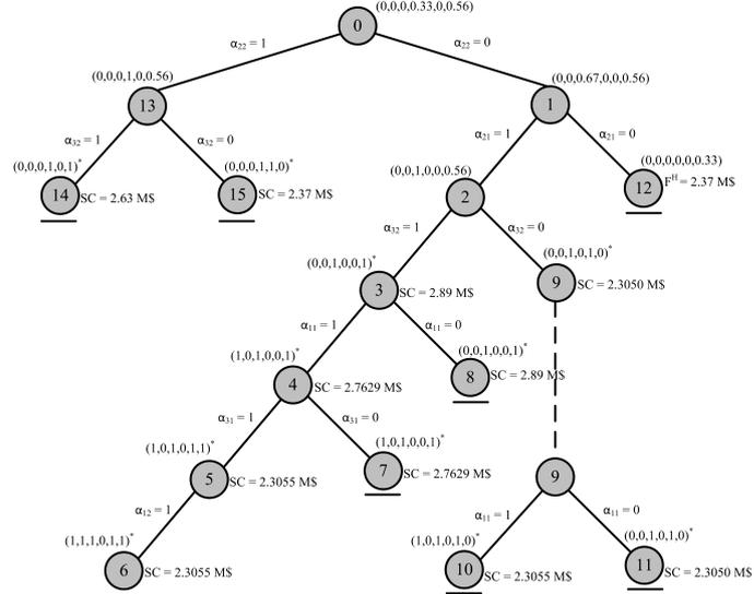
Figure 4.5: The branch-and-bound tree of the MBA for the 3-bus example system;  $(x,x,x,x,x,x)=(\alpha_{11},\alpha_{12},\alpha_{21},\alpha_{22},\alpha_{31},\alpha_{32}), \alpha \in \{0,1\}$ , SC: Social Cost.
