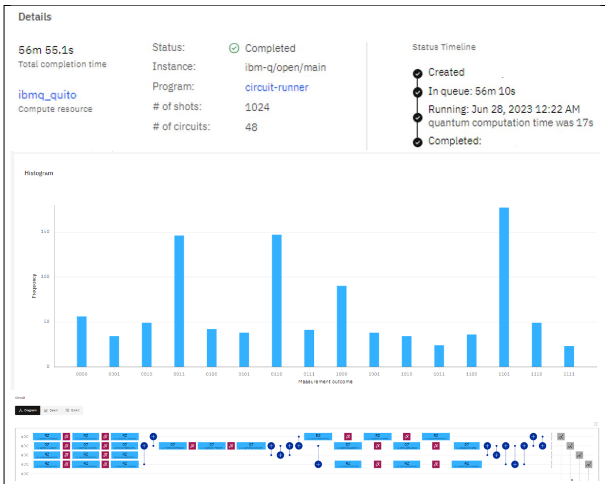
Figure 27 – IBM Quantum Platform screenshot showing for a random job: main characteristics: time, number of circuits & jobs; bar chart of frequency of measurements for shots & compiled circuit
