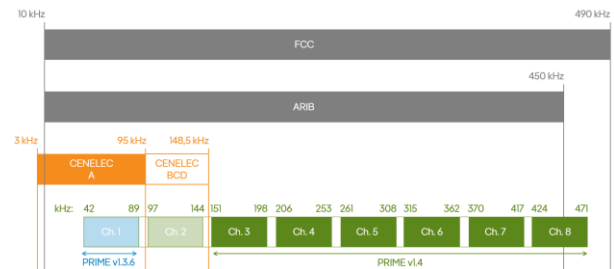
Figure 5: Frequencies band for NB-PLC. [Own preparation]
