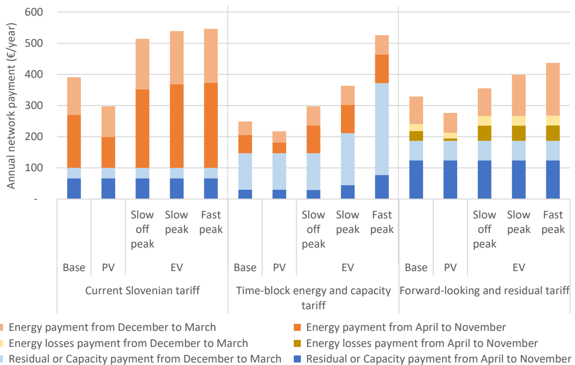
Figure 4.7. Network payments (€/year) for a representative LV customer household under each tariff design after installing PV or EV following three strategies: slow off-peak, slow peak, and fast peak. Source: (Morell-Dameto et al., 2023a)
