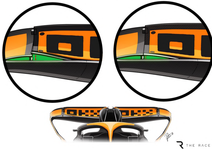
Figure 28: McLaren rear wing deflection at high speed.
