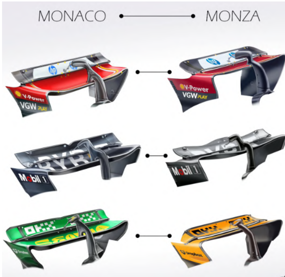
Figure 16: Rear wing configurations: Monaco (left, high downforce) vs. Monza (right, low drag).
