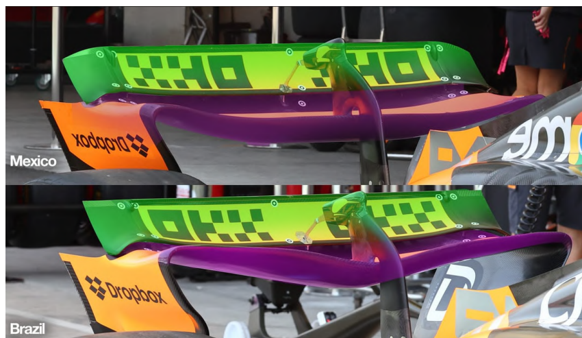
Figure 39: McLaren rear wing comparison between Mexico and Brazil during the 2025 races
