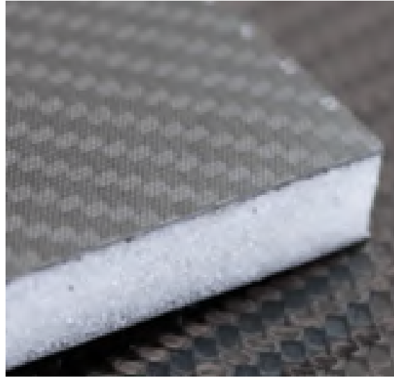
Figure 57: ROHACELL used as core
