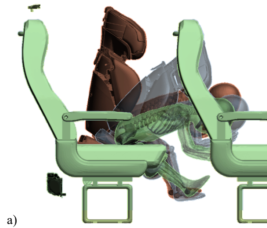
Figure 2. 3YO and 6YO PIPER HBM models (subfigures a and b, respectively) seated in the bus model in two configurations: 3P seatbelt with no Booster (orange) and with Booster (blue).
