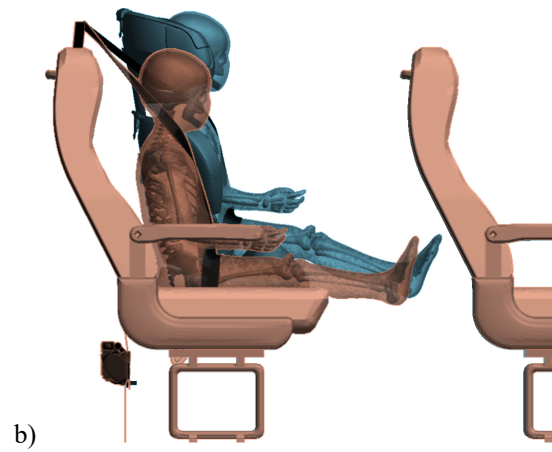
Figure 2. 3YO and 6YO PIPER HBM models (subfigures a and b, respectively) seated in the bus model in two configurations: 3P seatbelt with no Booster (orange) and with Booster (blue).
