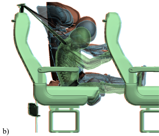
Figure 4. 6YO PIPER HBM excursion combined with no Booster (green), Booster (blue), and Booster+ISOFIX (orange) using a 2P seatbelt (shown at 150 ms) and a 3P seatbelt (shown at 100 ms).
