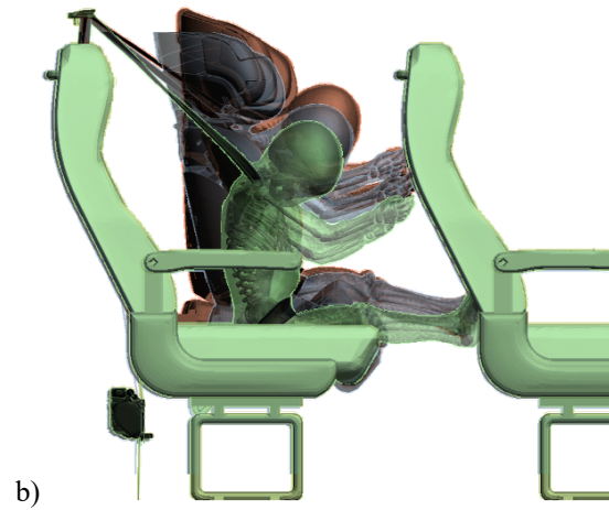
Figure 3. 3YO PIPER HBM excursion combined with no Booster (green), Booster (blue), and Booster+ISOFIX (orange) using a 2P seatbelt (top)) and a 3P seatbelt (bottom).
