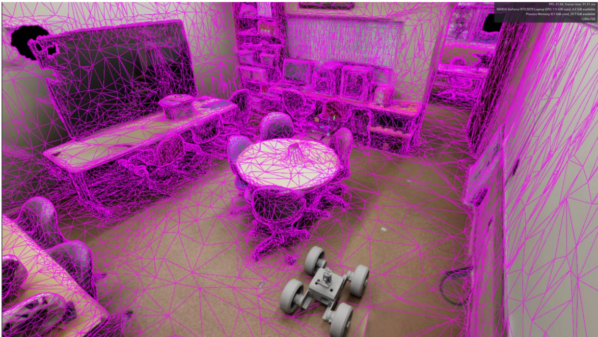
Figure 5. Photorealistic reconstruction of the laboratory and superposition of the 3D collision mesh indexed by PhysX in NVIDIA Isaac Sim (Source: Author).
