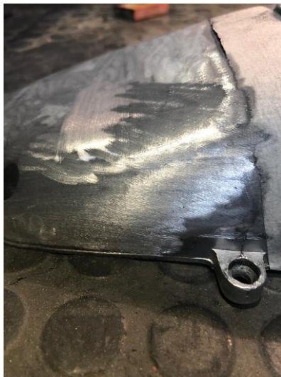
“defecto surco tras lija 80”
