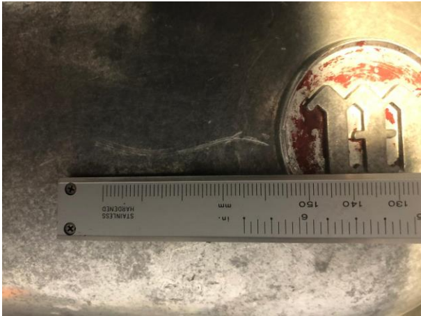
“defecto surco previo pulido”
