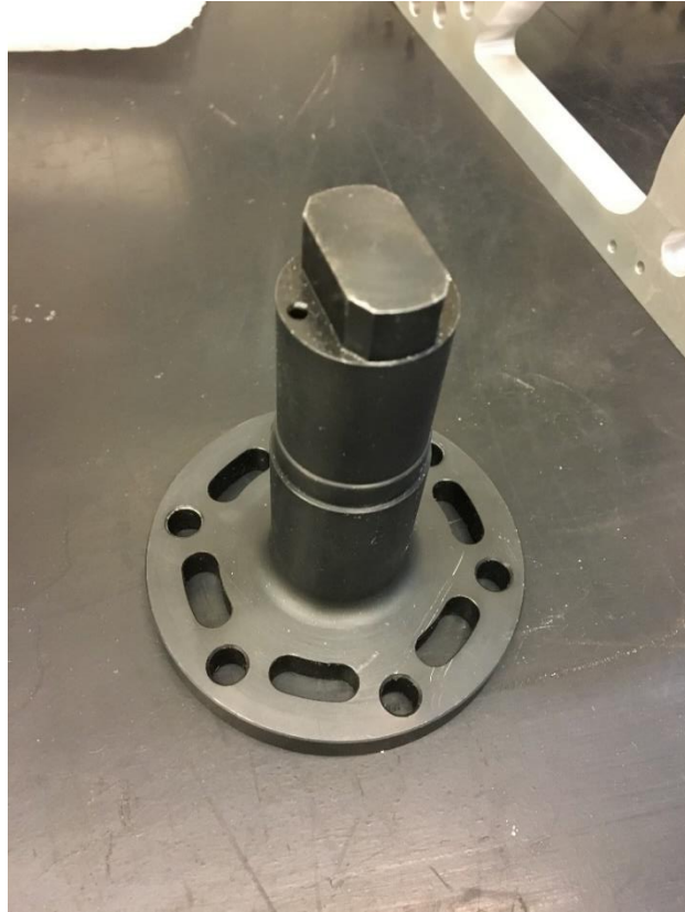
Figure 4: Output shaft of the motor manufactured
