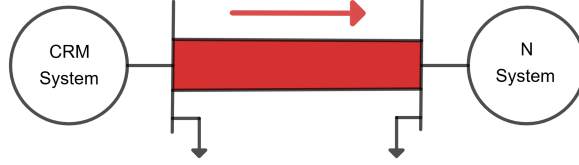
Figure 2: Case 2. P_{max}^{CRM-system} < P_{max}^{N-System}
