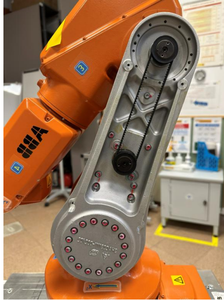
Figure 1. Structural arm of Link 2 (own elaboration)
