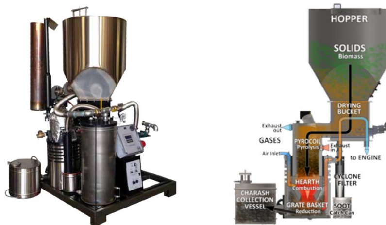
Figure 21: GEK gasifier: kit, processes and flows [25]
