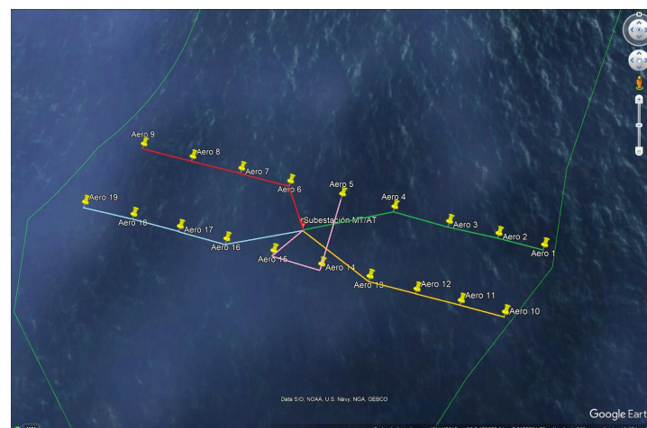
Figura 2. Design of the wind farm MV circuit (Google Earth).
