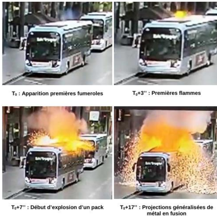
Figure 12: Chronological sequence of the thermal runaway in a Bluebus [BEAT23].
