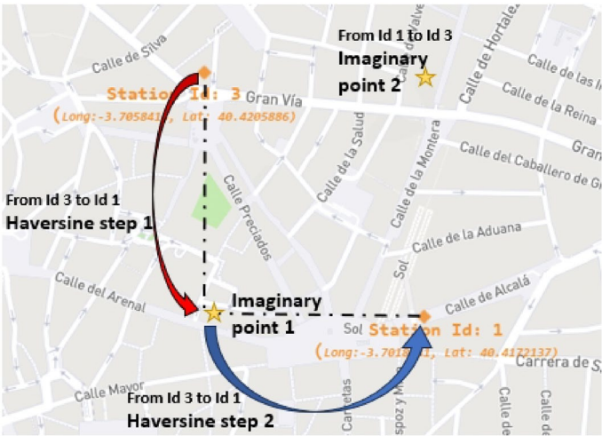
Fig. 6. Distance calculation based on a mix of Haversine and Mahattan.
