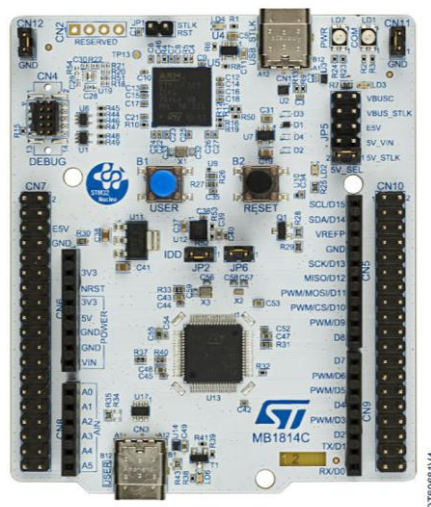
Figura 1: Placa de desarrollo STMicroelectronics STM32 Nucleo-64 H533RE
