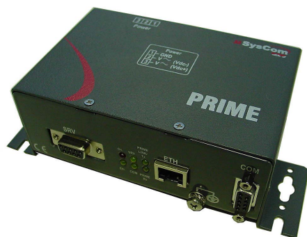
Figure 4: PRIME Base Node implementation
