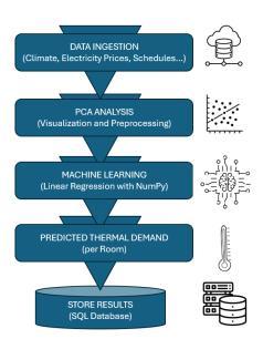
This module represents the intelligence of the system, focusing on data ingestion, preprocessing, prediction and decision-making. Implemented in Python, it leverages scientific libraries (NumPy, Pandas, Scikit-learn) and Machine Learning techniques to forecast both thermal demand and electricity prices fluctuations.
