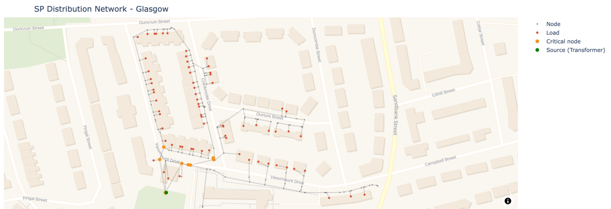
Figure 32: Highlighted Whifflet's network representation showing critical nodes and overestimated nodes
