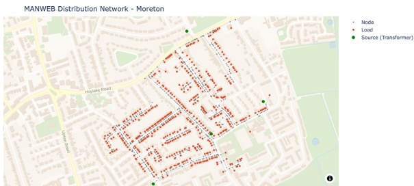
Fig. 5: Representation of the Moreton distribution network within SP area.
