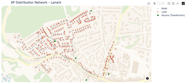
Fig. 3: Representation of the Lanark distribution network within SP MANWEB area.
