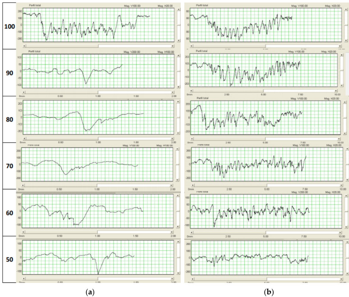
Figure A9. (a) One measurement on one line and (b) the black area for 1800 mm/min and different ranges of power from 50% to 100% of the laser.
