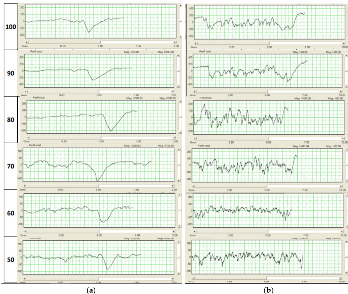
Figure A1. (a) One measurement on one line and (b) the black area for 1000 mm/min and different ranges of power from 50% to 100% of the laser.
