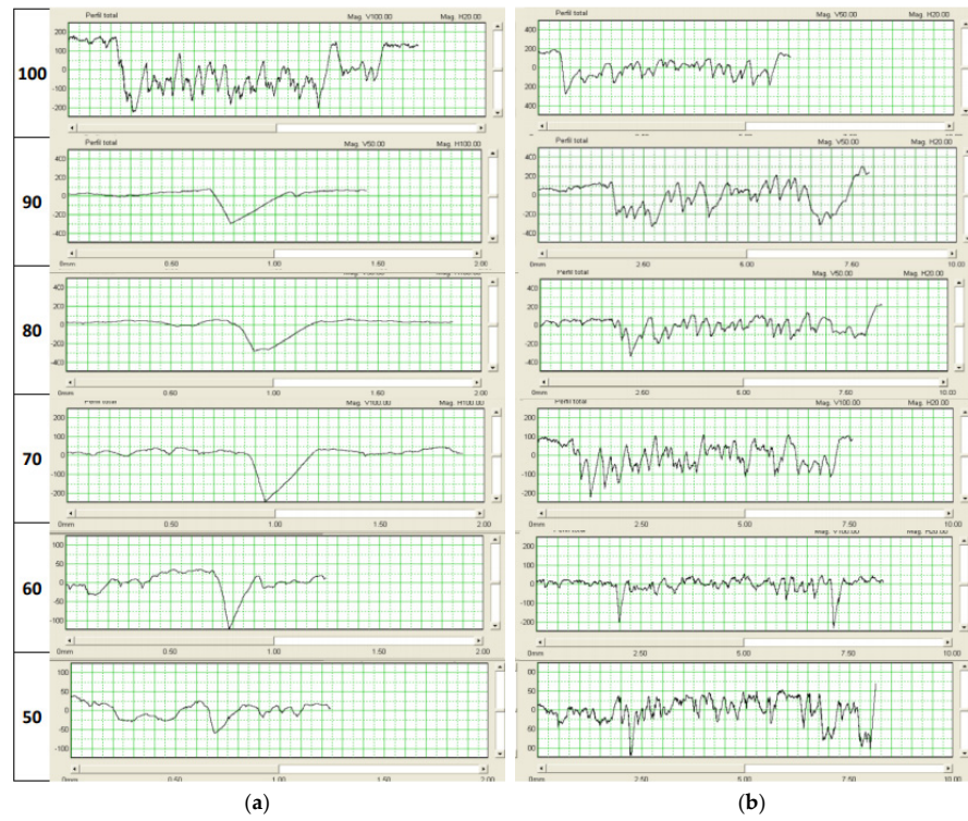
Figure A10. (a) One measurement on one line and (b) the black area for 1900 mm/min and different ranges of power from 50% to 100% of the laser.
