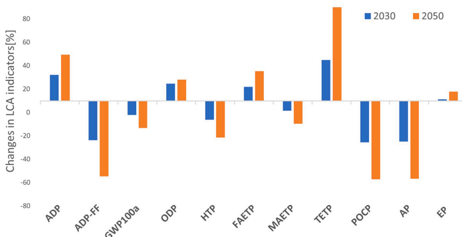
Fig. 4. Percentage changes in LCA results for clinker in the 2030 and 2050 scenarios compared to the 2021 baseline, across eleven evaluated impact categories.
