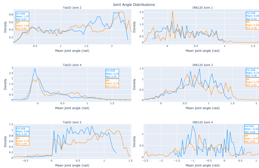
Figure 9. Joint angle distributions for the best full KGE agent (blue) and the best BM agent (orange), with DR. The first column corresponds to the TIaGO and the second to the IRB120. The selected joints for TIaGO are joints 2, 4, and 5, and for the IRB120, they are joints 1, 2, and 4.
