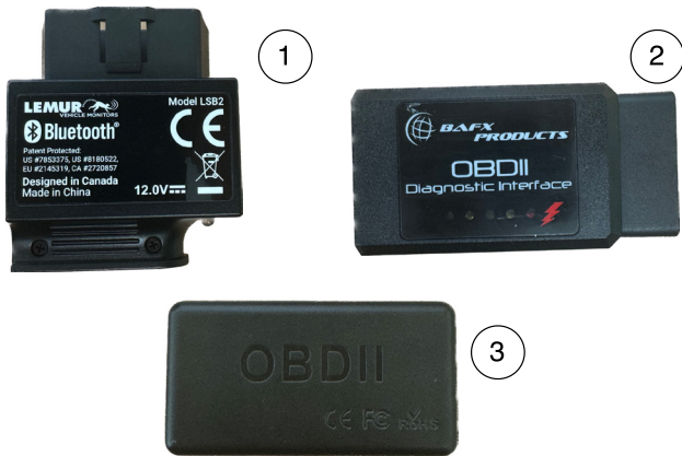
FIGURE 1. Examples of commercial OBD dongles: (1) BlueDriver (model LSB2) from Lemur Vehicle Monitors, (2) Bluetooth OBDII Reader from Bafx Products, (3) generic ELM327-compatible device.
