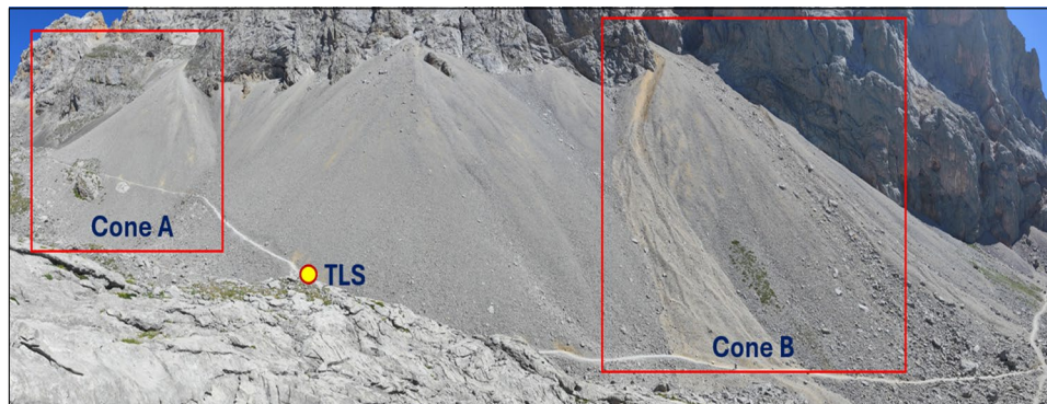
Fig. 2 Photograph of Cone A and Cone B including terrestrial laser scanning (TLS) station. The source area of debris cone material is the weathered and tectonically weakened limestone walls
