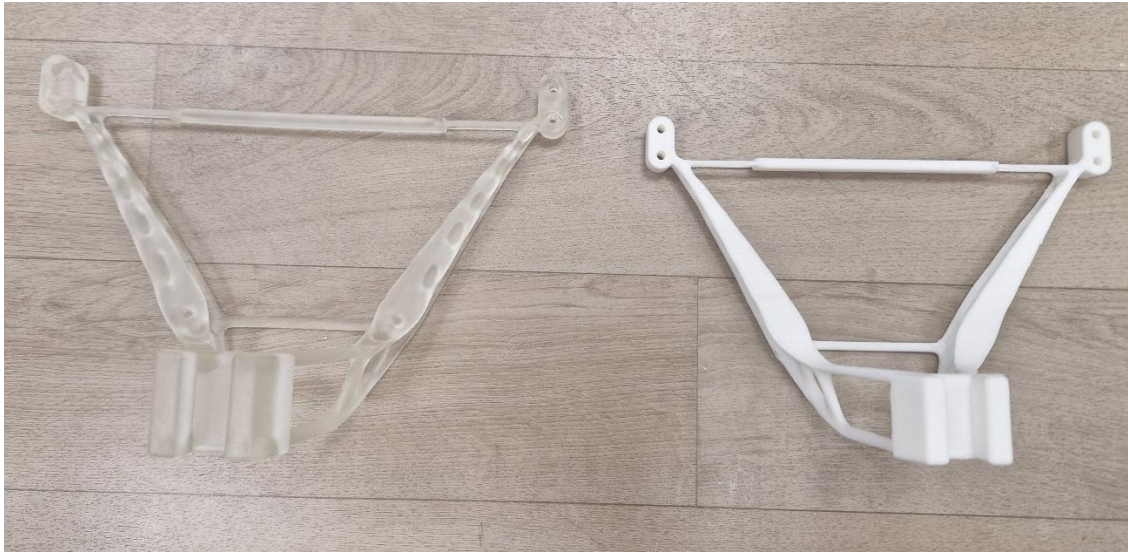
Ilustración 4: Optimised fairing stay printed in 3D
