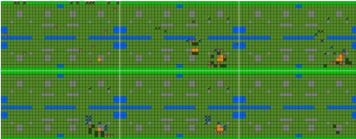
Figure 14: MAPPO at the publishable hard cell ( d=1.0 , N=10 , seed 42, run 7). Read left to right: the team spreads along the fire front, refills its finite water tanks in shifts, and converges on residual hotspots without crowding a single cell. The map is cleared in 69 steps and the per-agent returns are tightly bunched (between 63 and 67). That tight bunching is the per-episode behavioural signature of the well-distributed cooperation that, in aggregate, produces the 83.7% seed-averaged clearance at this difficulty (Section 6.4).
