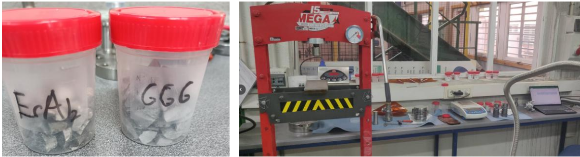
Figure 40 Pre-crushed particles of \text{ErAl}_2 and GGG (left) and laboratory set up during manufacturing (right), which includes the hydraulic press, a sieve, a high precision weight scale and a computer for data acquisition.
