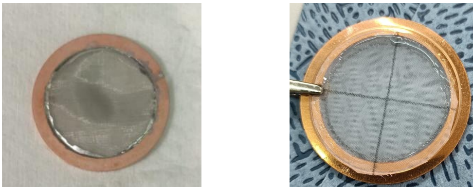
Figure 50. Copper gasket with soldered stainless-steel mesh for packed bed containment.
