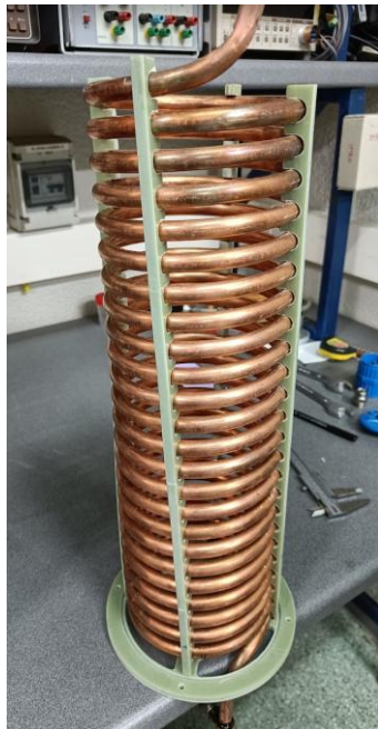
Figure 77. Heat exchanger as received with fiber glass separators (left), and heat exchanger assembled in cryostat (right)
