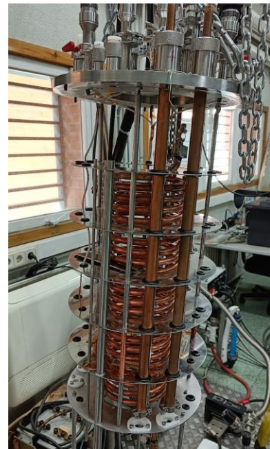
Figure 77. Heat exchanger as received with fiber glass separators (left), and heat exchanger assembled in cryostat (right)
