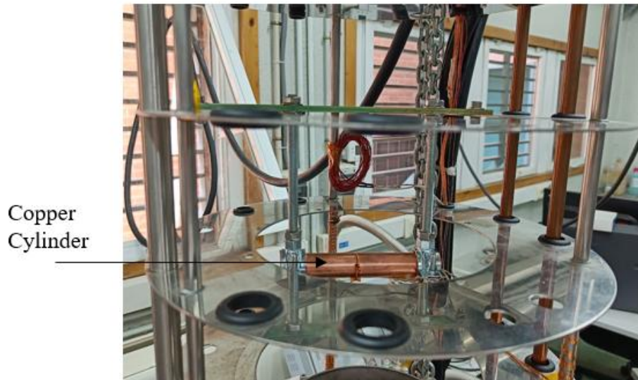
Figure 72. Placement of copper cylinder with heater for the evaluation of the heat transfer coefficient.
