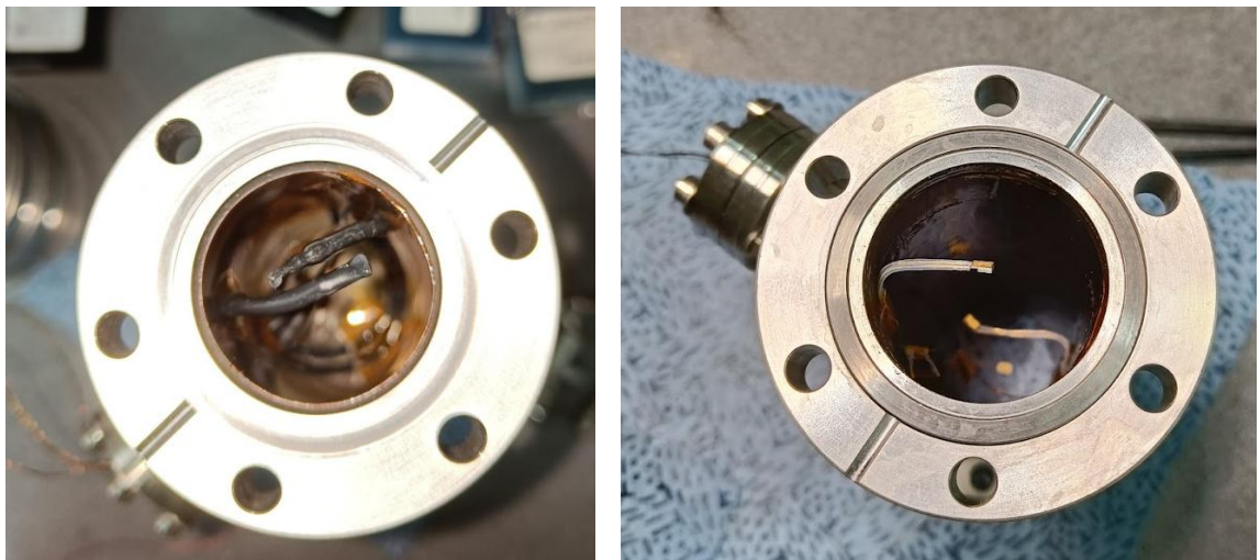
Figure 48. ErAl 2 and GGG packed bed housing with instrumentation placed before introducing the magnetocaloric material.
