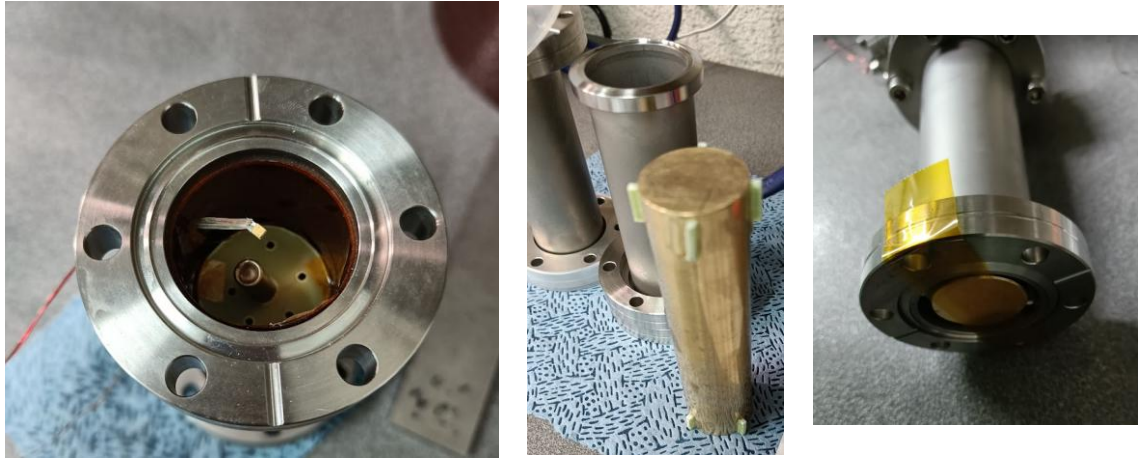
Figure 51. Stainless steel housing with heater and temperature sensor in place (left), brass block introduced inside stainless steel housing before entering the heater recipient (center and right).
