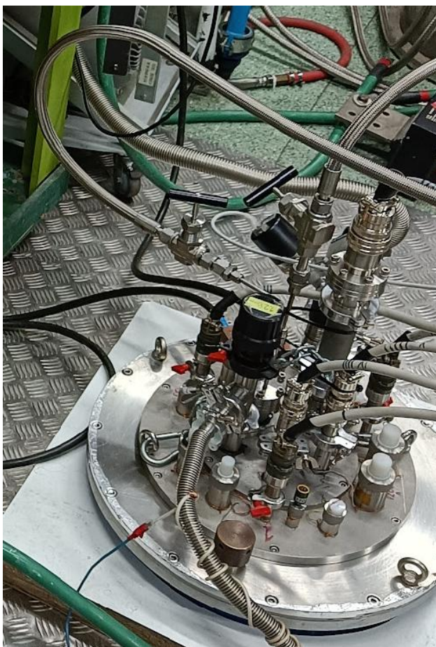
Figure 92. Upper view of the cryostat showing the cryogenic transfer lines and the manual valves used for changing the flow direction.
