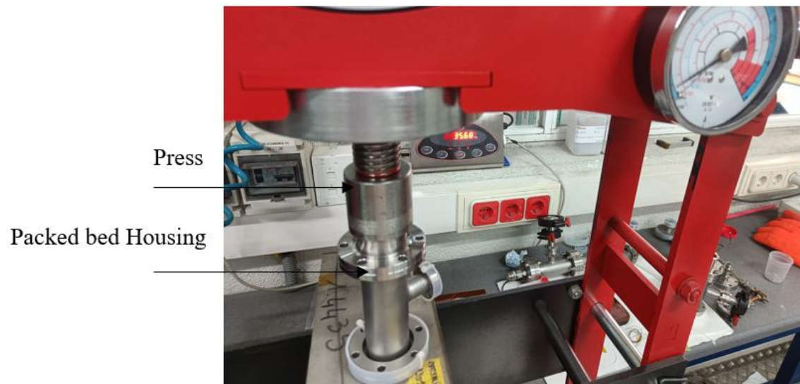
Figure 42. Application of pressure to the packed bed to achieve desired porosity.
