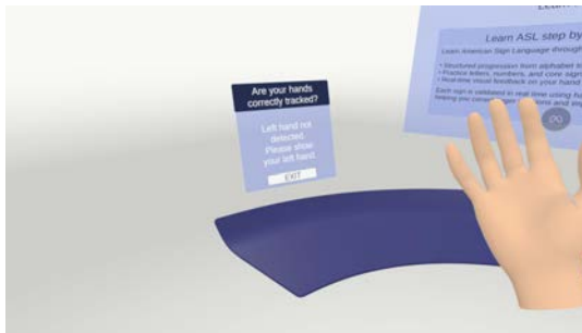
(c) Only right hand detected: the system indicates that the left hand is missing.
