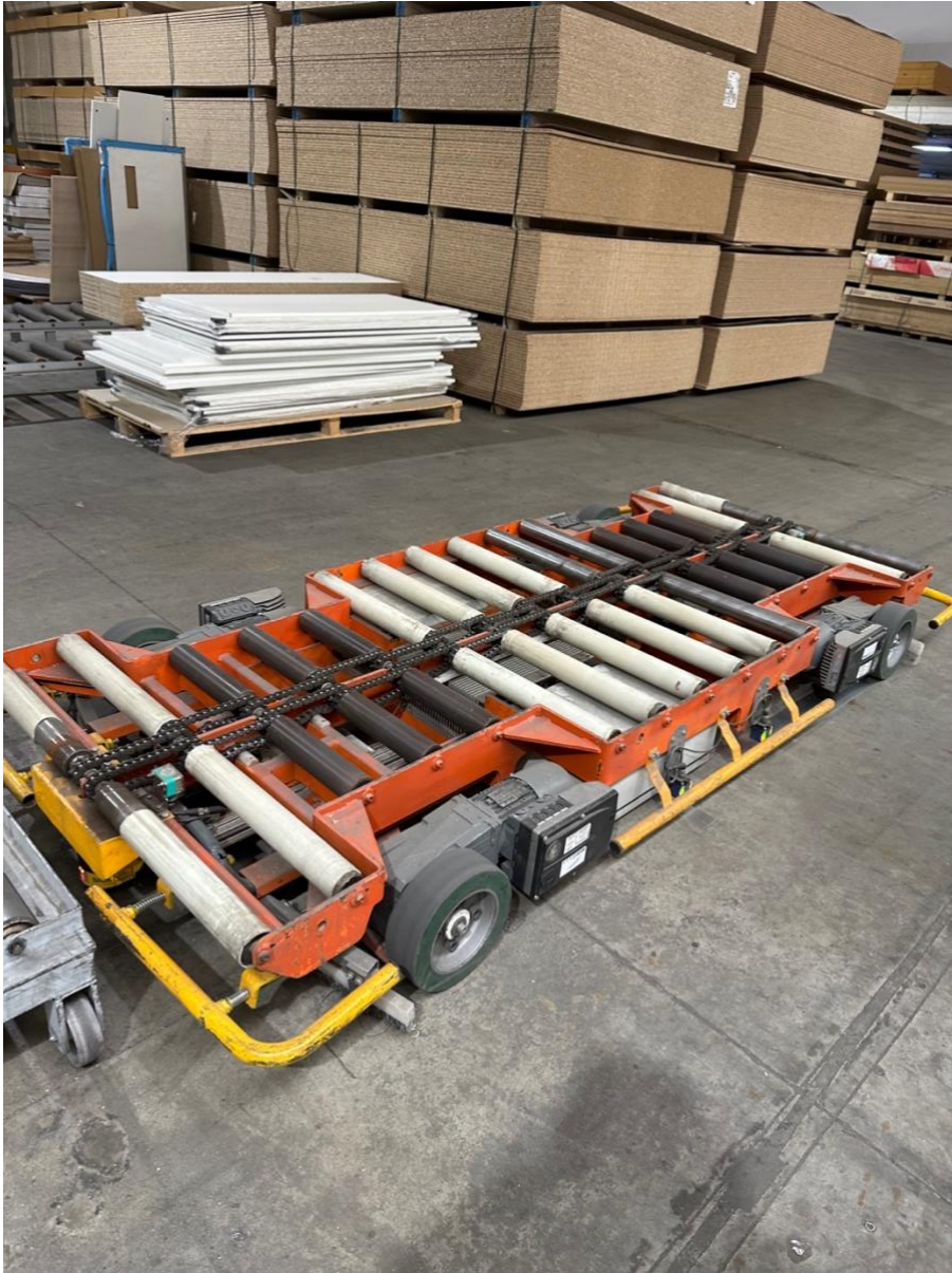
Photo 2. Automated guided vehicle that transports materials or products between areas
