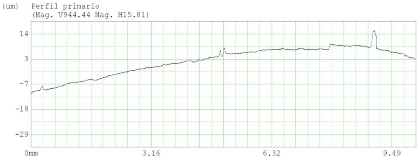
Figure A12. Primary profile; diagonal 3 before wear in sample E2.
