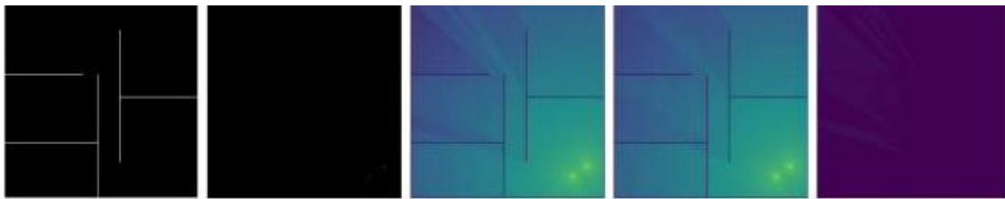
Figure 2. Qualitative example with the input floor plan and mask, the simulated map, the model prediction and the error.
