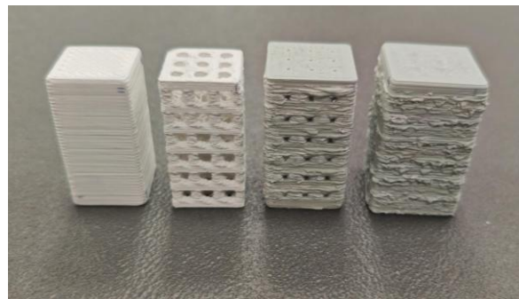
Fig. 10. 3D-printed scaffold prototypes (from left to right): bulk, porous SenScaffold, and SenScaffolds with 1 mm and 1.5 mm HA layers.
