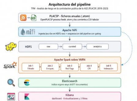
System architecture: layered pipeline with NiFi orchestration.
