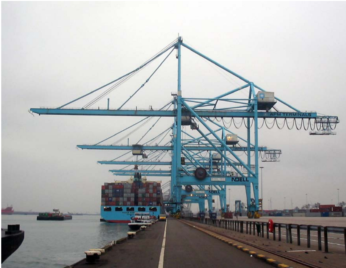
Fig. 3.2: Ship-to-Shore gantry crane
