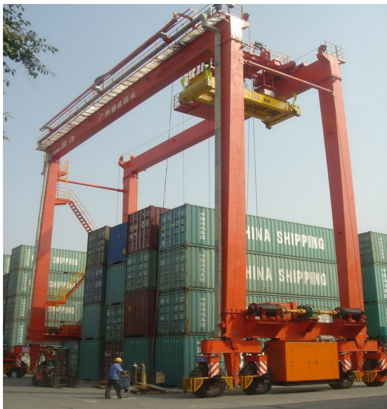
Fig. 3.8: Rubber Tyre Gantry Crane
