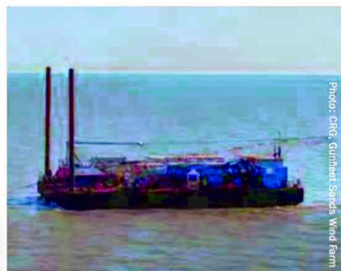
Floating dumb barge with crane
