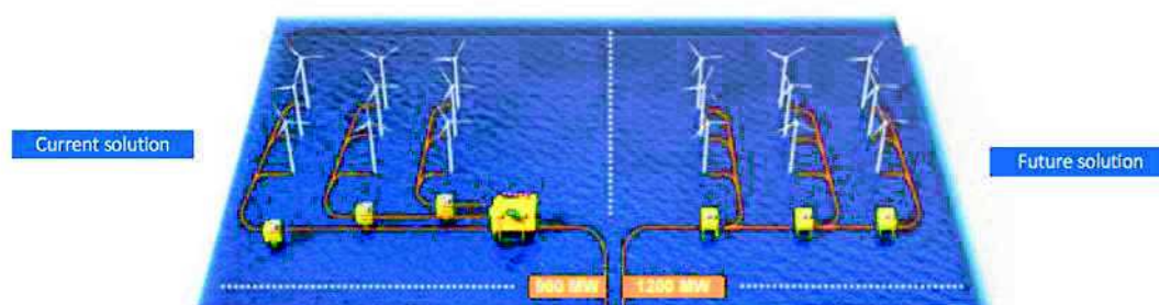
Figure 4.13 Siemens Grid Access using Diode Rectifier Units (SGA-DRU) HVDC solution. Source: 4C Offshore.
