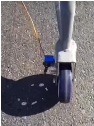
Figure 27. Servo in 70 degrees position (locked)
