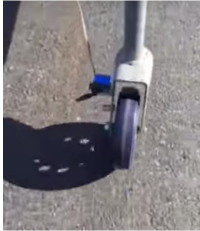
Figure 26. Servo in 30 degrees position (unlocked)
