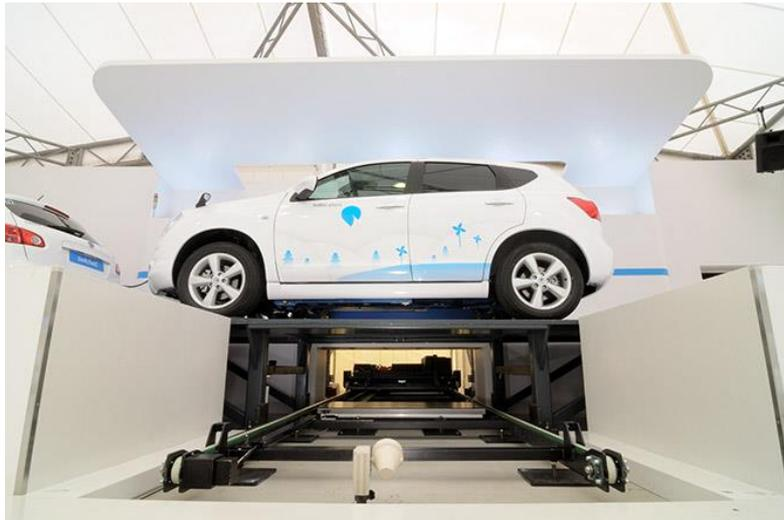
Fig. 56: Replacement of batteries in an electric car [28]
