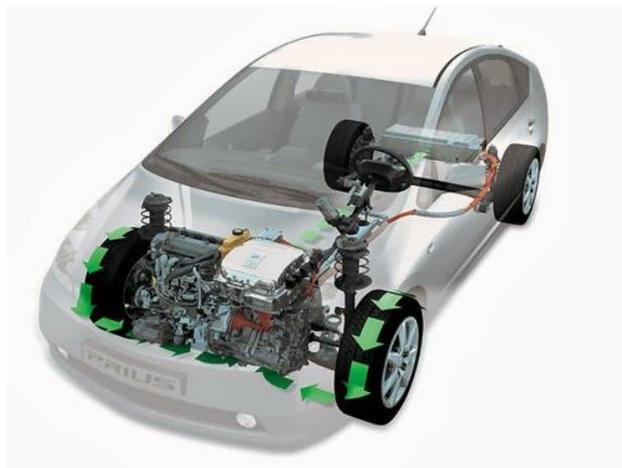
**Fig. 72:** Car with a regenerative brake [34]
