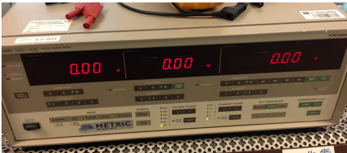
Figure 16. Digital Power Meter.
