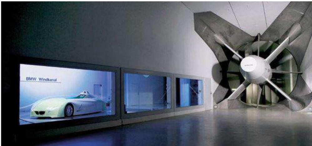
Ilustración 2.89 Ventilador. Fuente: [http://www.f1aldia.com/photos/10600/10650/001\\_small.jpg](http://www.f1aldia.com/photos/10600/10650/001_small.jpg)
