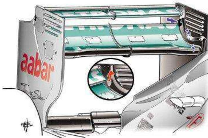
Ilustración 2.51 S-Duct Mercedes. Fuente: [http://2.bp.blogspot.com/-m5zk\\_rELGM/T26k0xYKTJ/AAAAAAAAEV8/4RysdK1inAc/s1600/S-Duct+Mercedes+W03.jp](http://2.bp.blogspot.com/-m5zk_rELGM/T26k0xYKTJ/AAAAAAAAEV8/4RysdK1inAc/s1600/S-Duct+Mercedes+W03.jp)
