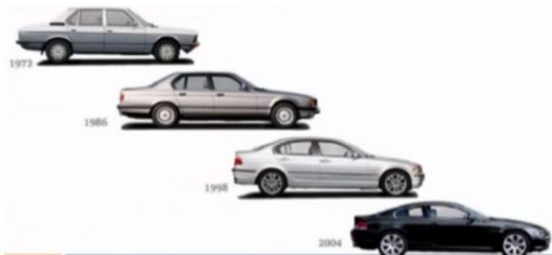
Figure 1–6 - Aerodynamic design evolution of an example road car, in this case the BMW.
