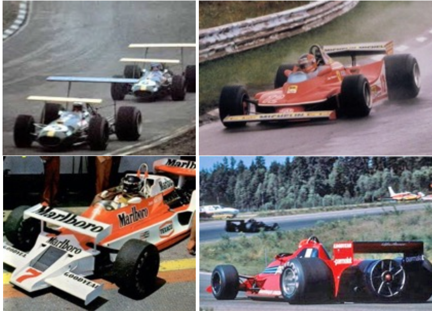
Figure 1–5 - Examples of disruptive designs in Formula 1, either because of the wing design, or the nose design, or even the introduction of a fan for increased downforce.
