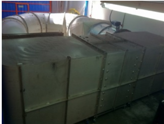
Figure 6–14 – Prototype wind tunnel for testing purposes presented to validate the CFD solver used.
