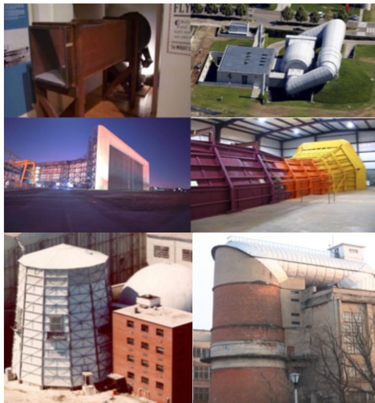
Figure 4–1 - Different types of wind tunnels. From right to left and top to bottom: Replica of the Wright wind tunnel; Closed wind tunnel at the Ferrari Formula 1 Team; Open wind tunnel at NASA Ames Research Center; A2 open wind tunnel for testing of various kinds (including vehicles and professional cyclists and skiers); and vertical wind tunnels for scientific testing of aircraft spins, helicopter blades, and parachutes: at NASA Langley Research Center (first ever built vertical wind tunnel, 1940) and the TsAGI Vertical Wind Tunnel T-105 in Russia (1941).
