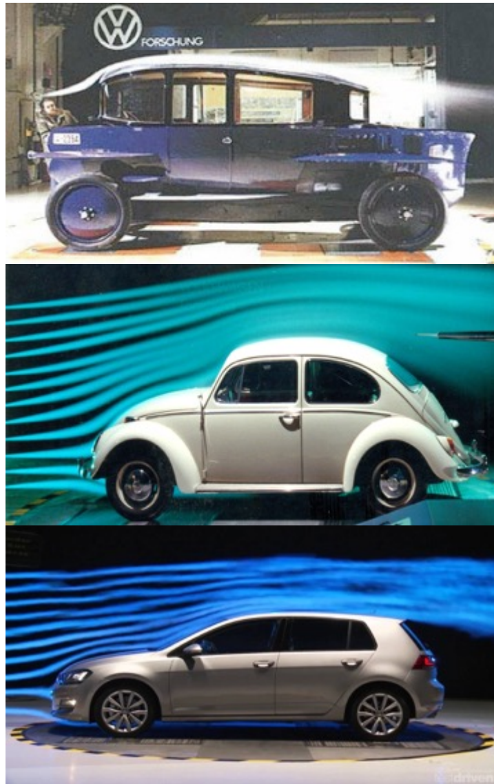
Figure 1–11 - Wind tunnel testing for three VW cars of different years. Velocity streamlines are simulated with a smoke generator. Changes in the flow field can be observed between the different car models.
