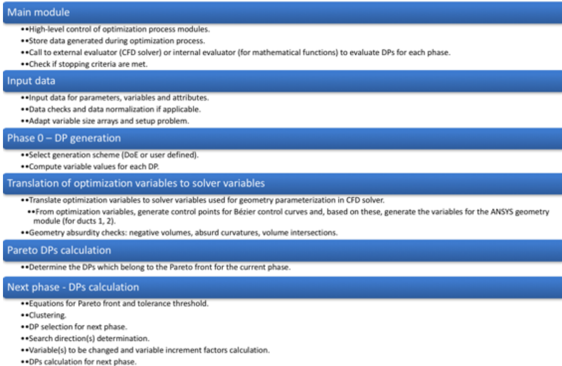
Figure 5–11 - Schematic diagram of the module architecture of the MOST-HDS model implementation for a fully automatic optimization workflow, coupling Microsoft Excel VBA and an external solver or evaluator, if required (in this case ANSYS was used for the CFD evaluations).
