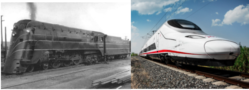
Figure 1–7 - Aerodynamic design evolution in the train sector. A steam high speed train, capable of maximum speeds of 160km/h and average speeds of 130km/h, compared to the most modern Talgo train, the Avril, capable of maximum speeds of 363km/h and average speeds of 330km/h.
