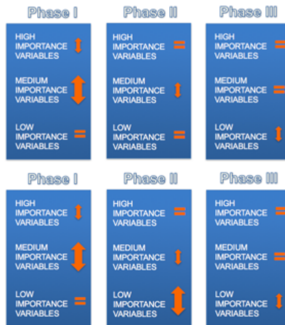
Figure 5–1 - Optimization model structure, illustrating the optimization phases, for two example set-up configurations. The arrows and equal signs indicate magnitude of change for each type of variable in each phase.
