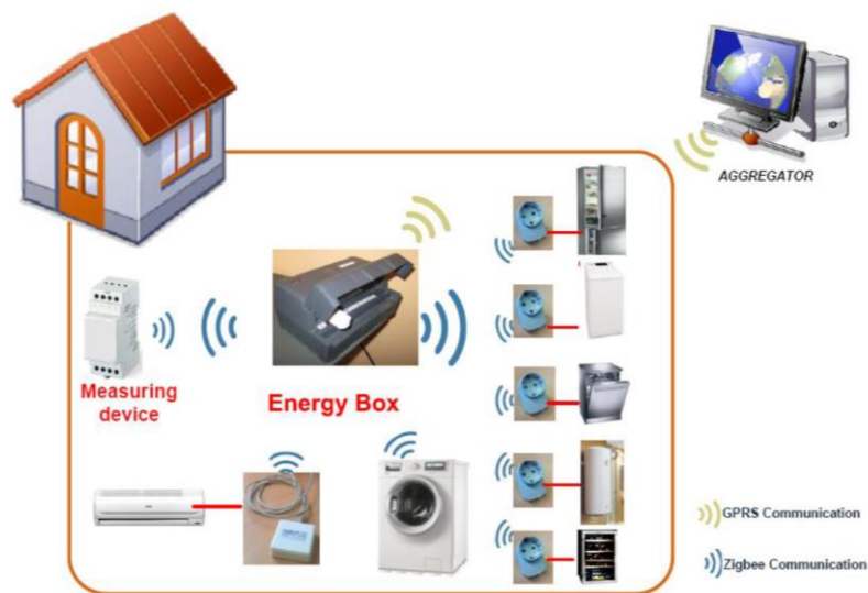
Figure 2.7. Schematic representation of a fully equipped home in the pilot program. Source: (Caujolle et al., 2011).
