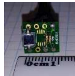
Figure 4. PPG sensor with photodiode (left) and dual LED (right)
