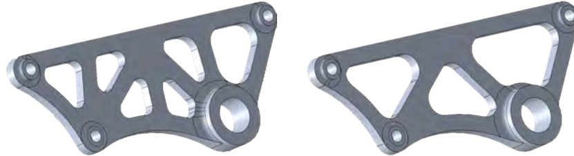
Figure 5.19: RBC design configuration
