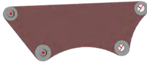
Figure 5.15: Solid Thinking Inspire refined design space
