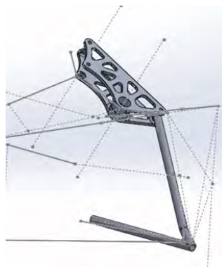
Figure 5.23: Rear Bellcrank system model
