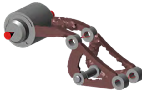
Figure 5.33: Front bellcrank topological optimization
