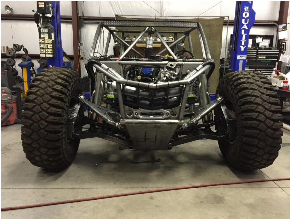
Figure 15: Double wishbone suspension truck
