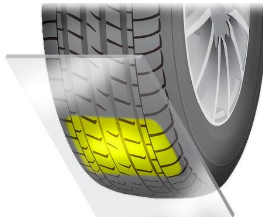
Figure 19: Contact surface tyre-ground
