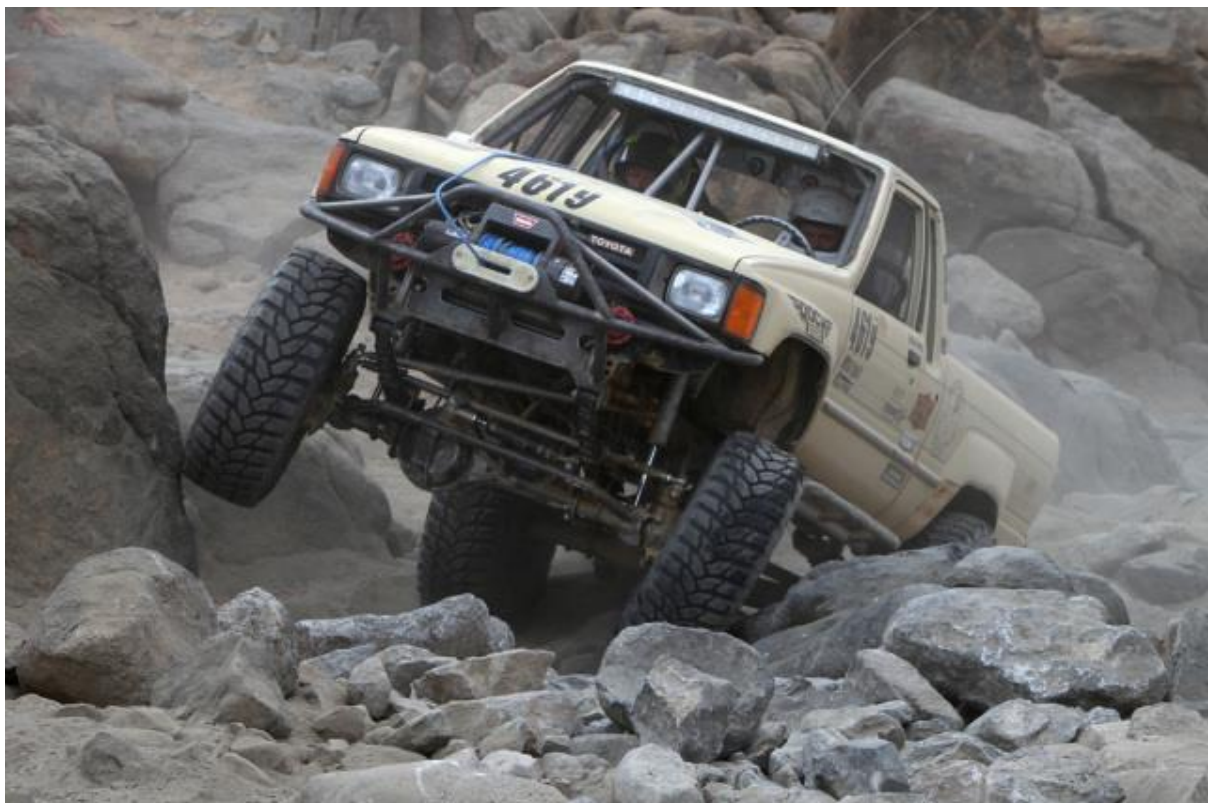
Figure 12: Solid axle suspension truck
