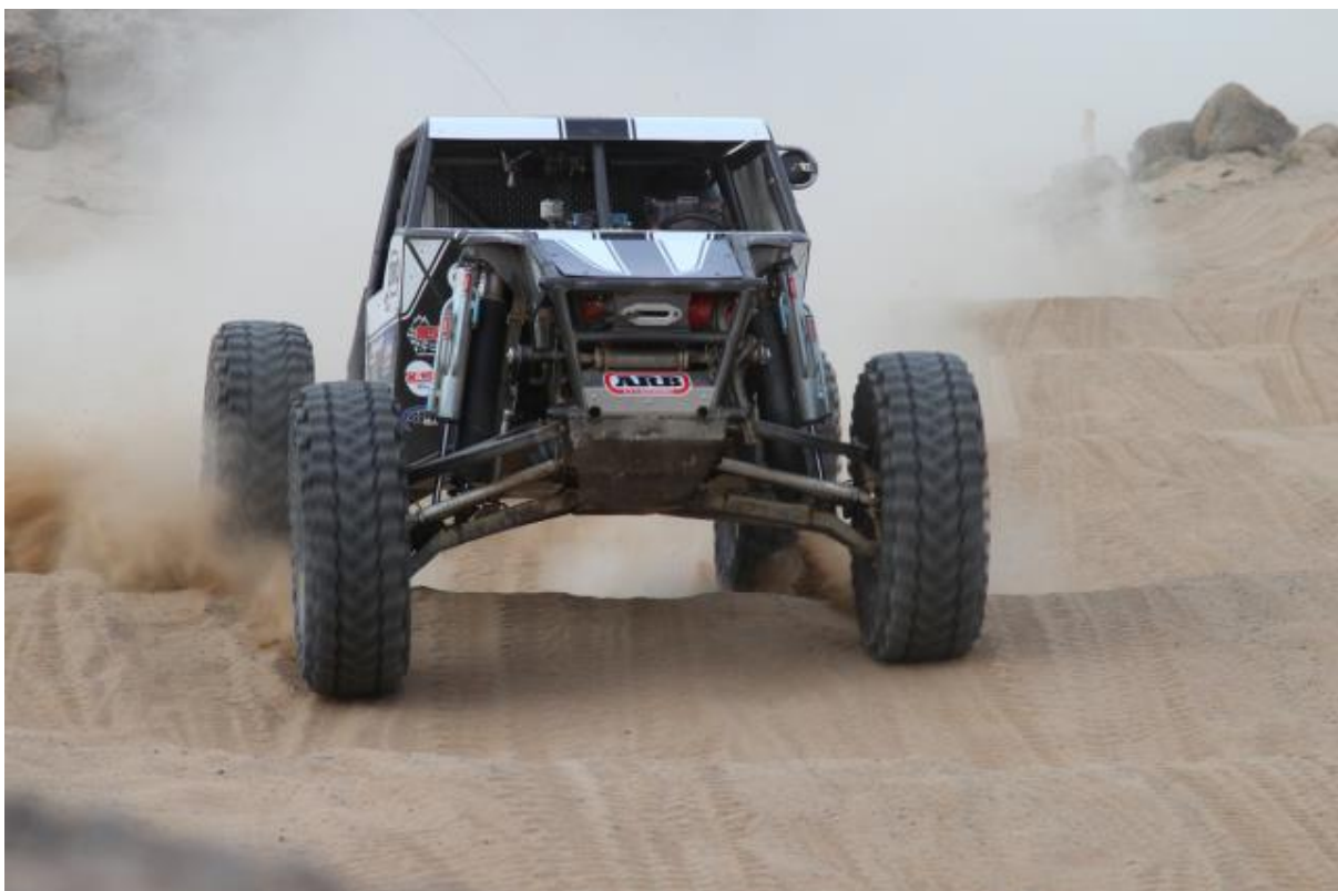
Figure 14: Fully independent suspension truck
