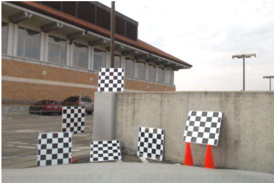
Figure 6: LIDAR-Camera KITTI Calibration Checker Board Setup
