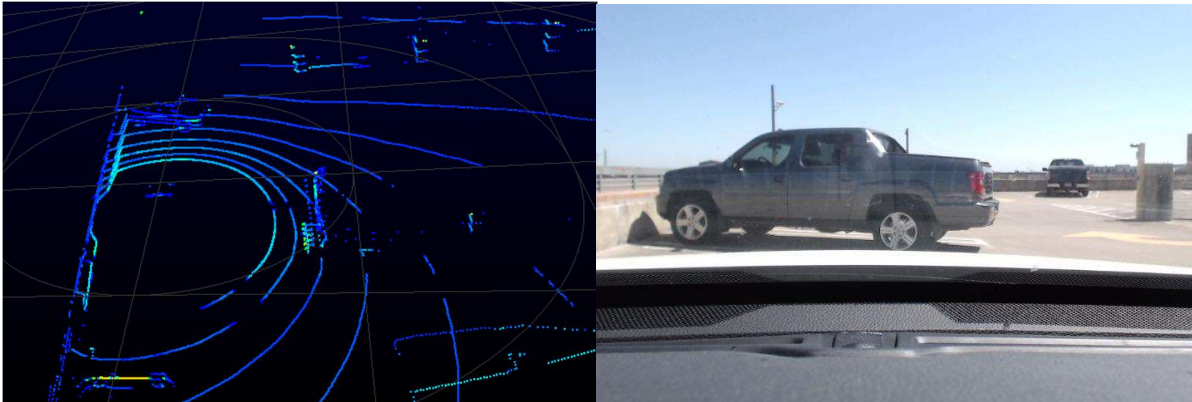
Figure 8: Point Cloud (Left) and Photo (Right) of Truck LCT setup
