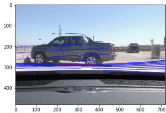
Figure 9: Image of point cloud overlaid on truck using LCT
