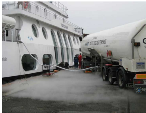
Figure 2 - TTS bunkering Source: Cryo AB
