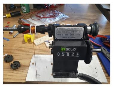
Figure 4.1. Process of winding a coil for the inductor  $L_2$ .
