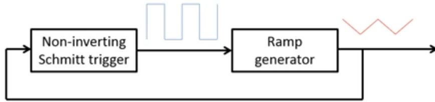
Fig. 3.16 Block diagram for generating triangular wave
